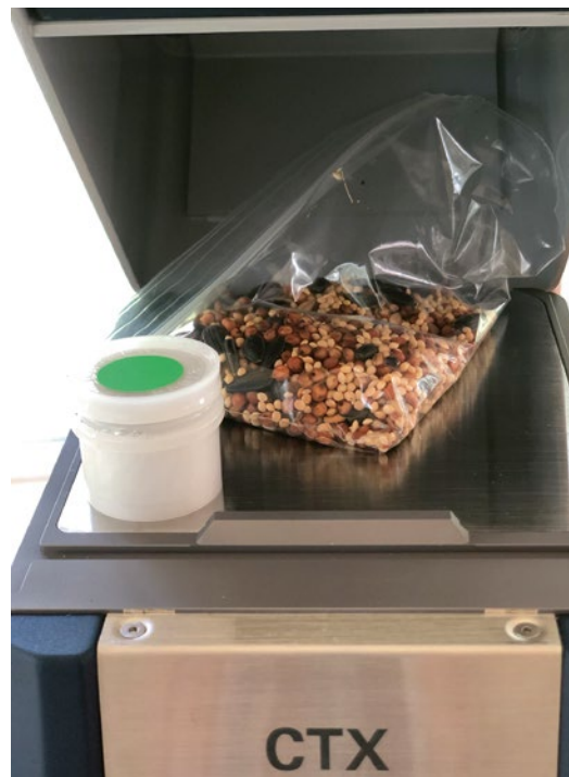
The CTX is a portable benchtop spectrometer and pre-calibrated to measure elements for a given application.
