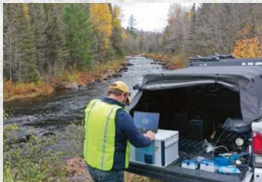
Field measurement with the S2 PICOFOX TXRF spectrometer without any need of lab equipment.
