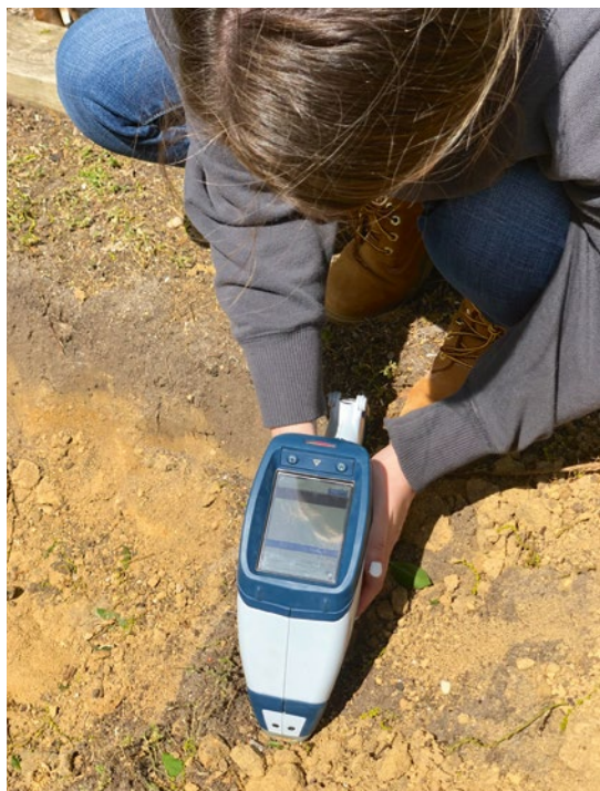
Handheld XRF spectrometers like the S1 TITAN are used to quickly screen soil for minerals and toxic metals.
