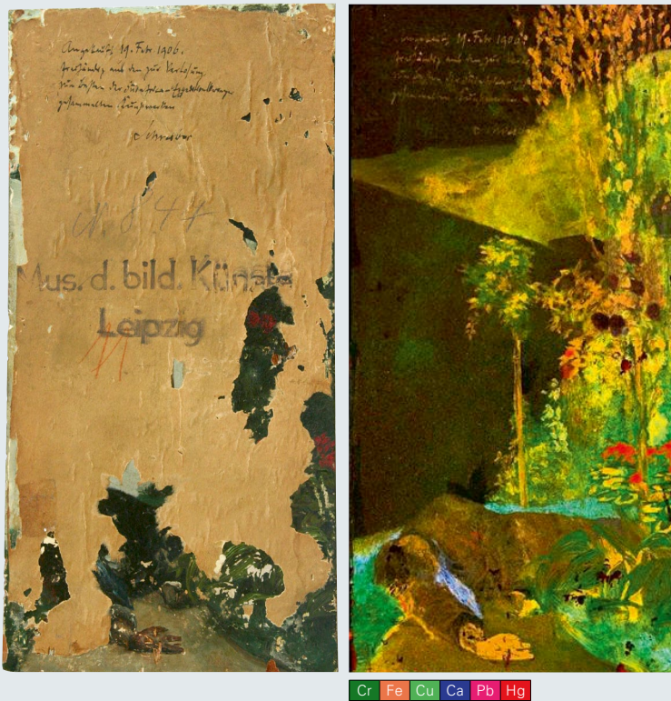
Left – Backside of a painting by Max Klinger (1872, approx. 14,5 x 32 cm 2 ) on a piece of wood (approx. 8 mm thick) covered with paper. Right – A hidden painting is “uncovered” by multi-element distribution analysis: the distribution of Cr, Fe, Cu, Ca, Pb and Hg, contained in pigments used, produces a false-color representation of the picture.
