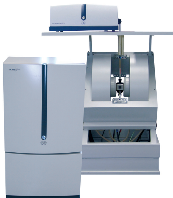
The EMXplus can be used for CW-ENDOR and Teslameter experiments
