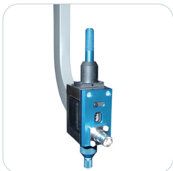
Dielectric resonator for very small (3mL) sample volumes
