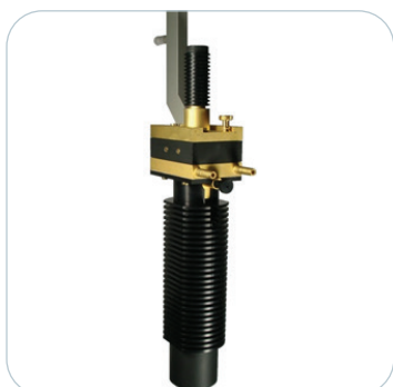
High Temperature resonator up to 1200 K
