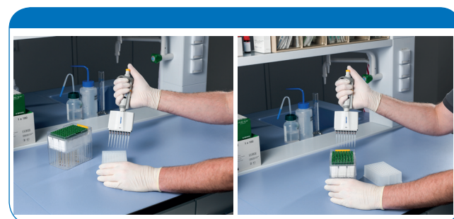
The SampleJet's 96 tube rack is compatible with sample preparation using standard liquid handling equipment.
