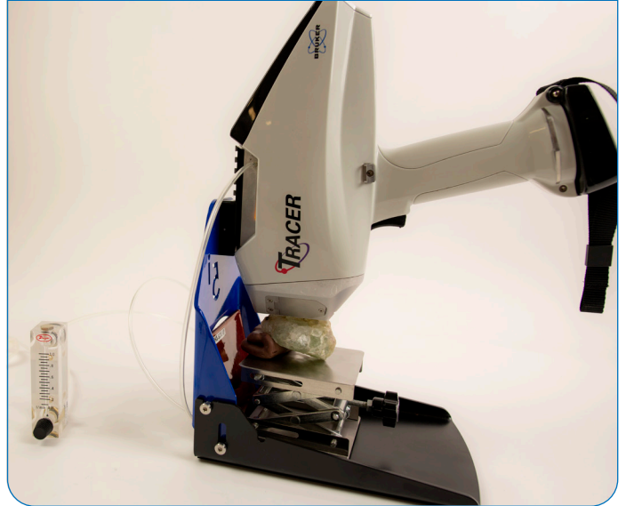
Figure 13: Molding clay used to help level the measurement surface
