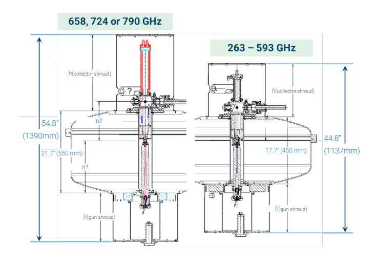
Cross-sectional view of Gyrotrons for up to 1.2 GHz (left), only 20 cm taller in the magnet stand and with matching diameter and footprint vs. to the 400 – 900 MHz family (right).
